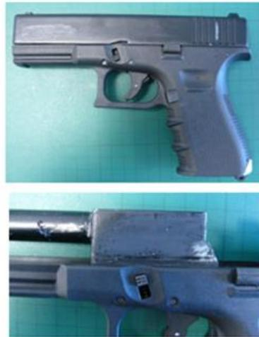
**Example of a modified Retay G17 with a replacement barrel and painted slide**
